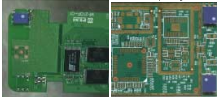
IEEE 802.11b WLAN Cards with Phycomp Antenna
